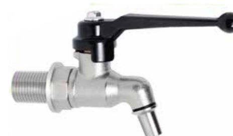
Corpo ottone nichelato- sfera ottone cromato-sedi PTFE-maniglia alluminio verniciato nero - codolo smontabile in ottone nichelato Corps laiton nickelé - boule laiton chromé - sièges PTFE - poignée en aluminium laqué noir - Avec queue démontable en laiton nickelé Nickel-plated brass body, chrome-plated brass ball, PTFE seats, black painted aluminium handle - demountable nickel-plated brass shank
