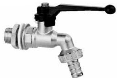
Corpo ottone nichelato- sfera ottone cromato-sedi PTFE-maniglia alluminio verniciato nero - portagomma e ghiera in ottone nichelato Corps laiton nickelé - boule laiton chromé - sièges PTFE - poignée en aluminium laqué noir - Douille et écrou en laiton nickelé Nickel-plated brass body, chrome-plated brass ball, PTFE seats, black painted aluminium handle - nickel-plated brass hose-end fitting and ring nut
